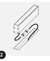
Make power connection to suit IP requirements of installation location. Insert MOMO-F Power.
