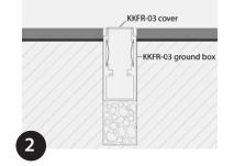
Line slot with butyl membrane if required. Drill for drainage holes in ground box and cable access hole if required. Position ground box on gravel, or permeable medium to set height to finished floor surface.
