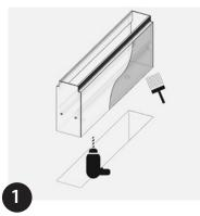
Drill for power cable entry (10mm/ 0.39" min). Coat aluminium box against corrosion if required. Install KKFR-03 ground box in floor slot and level to finished floor surface.
