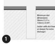
Cast slot from shuttered or solid form to suitable dimensions. If base of slot is not permeable additional drainage may be required.
